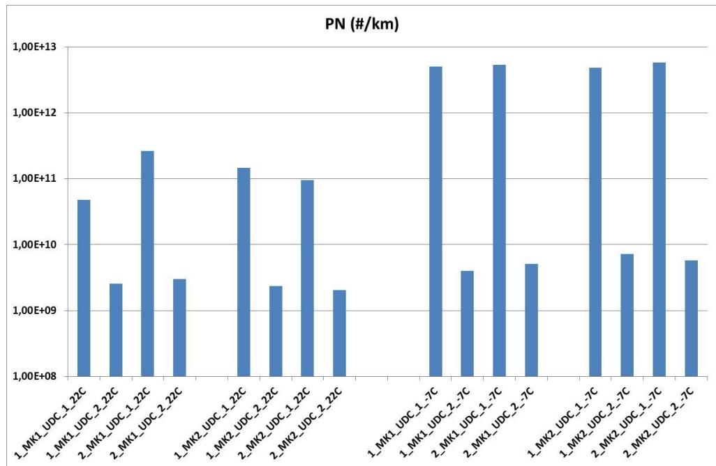
There are no significant differences in emissions of number of particles between the two fuels used. The number of particles is higher with start at low ambient temperature but the behaviors are same for both fuels. After reaching full catalytic activity the number of particles is about (# 3-5 +E9 per km).
