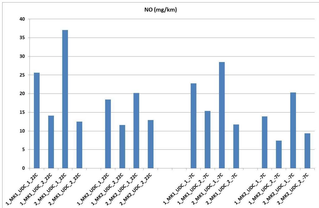
Interesting to note is that almost all NO<sub>x</sub> consists of NO (for modern diesel vehicles NO<sub>x</sub> consist mostly of NO<sub>2</sub>). There are no significant differences between use of MK1 and MK2.
