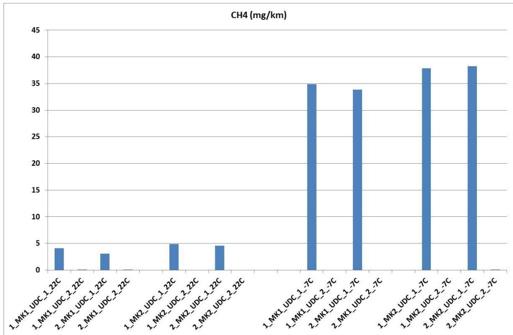
The emission of methane seems to be a little higher by using gasoline MK2 compared with MK1. But the differences are small and after reaching catalytic activity the emissions are close to zero for both MK1 and MK2. So the conclusion is that there are no differences in emission of methane with respect to the use of MK1 or MK2.
