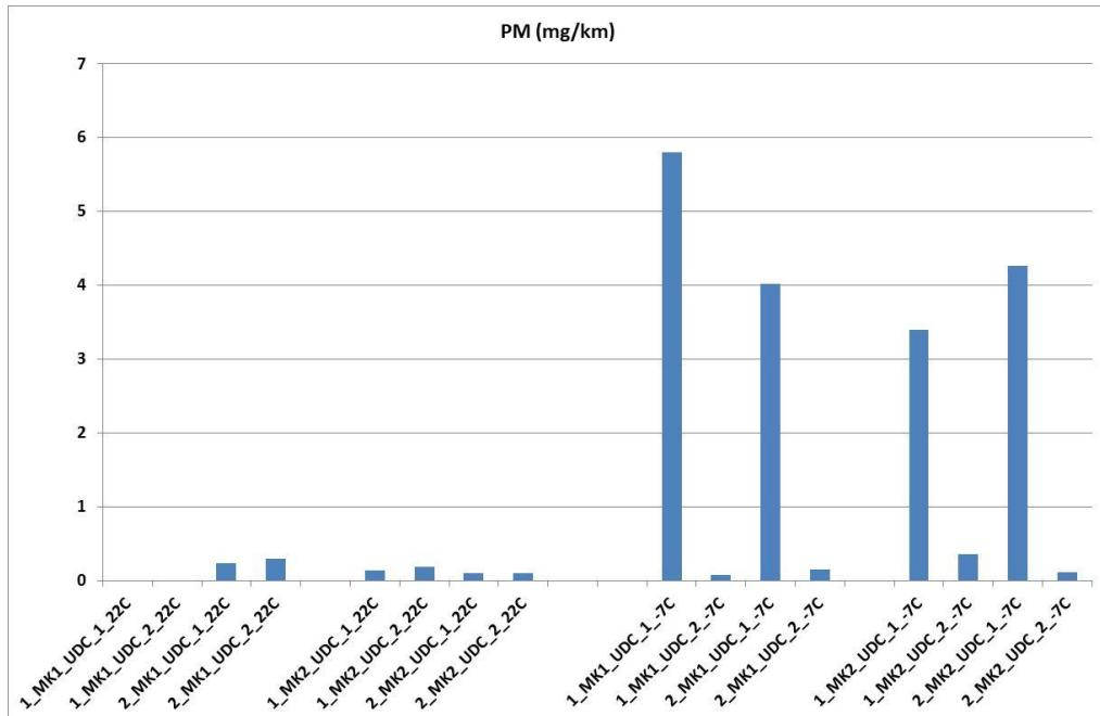
PM was measured by collecting particles on filter paper. These are very low weights (in absolute terms). This allows the measurement uncertainty is relatively large, so large that it is difficult to draw relevant conclusions from filter weight. A general conclusion is that there are very low PM emissions and that it is not any differences due to the use of fuel MK1 or MK2.
