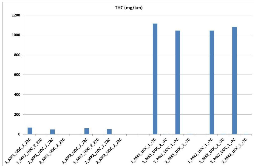
The emissions of hydrocarbons show no differences between gasoline of MK1 and MK2. For both gasoline's the emissions are higher with start at lower ambient temperatures. Higher cold start emissions due to longer time to reach catalytic activity at lower temperatures, but after reaching catalytic activity the emission of THC is close to zero thereafter.
