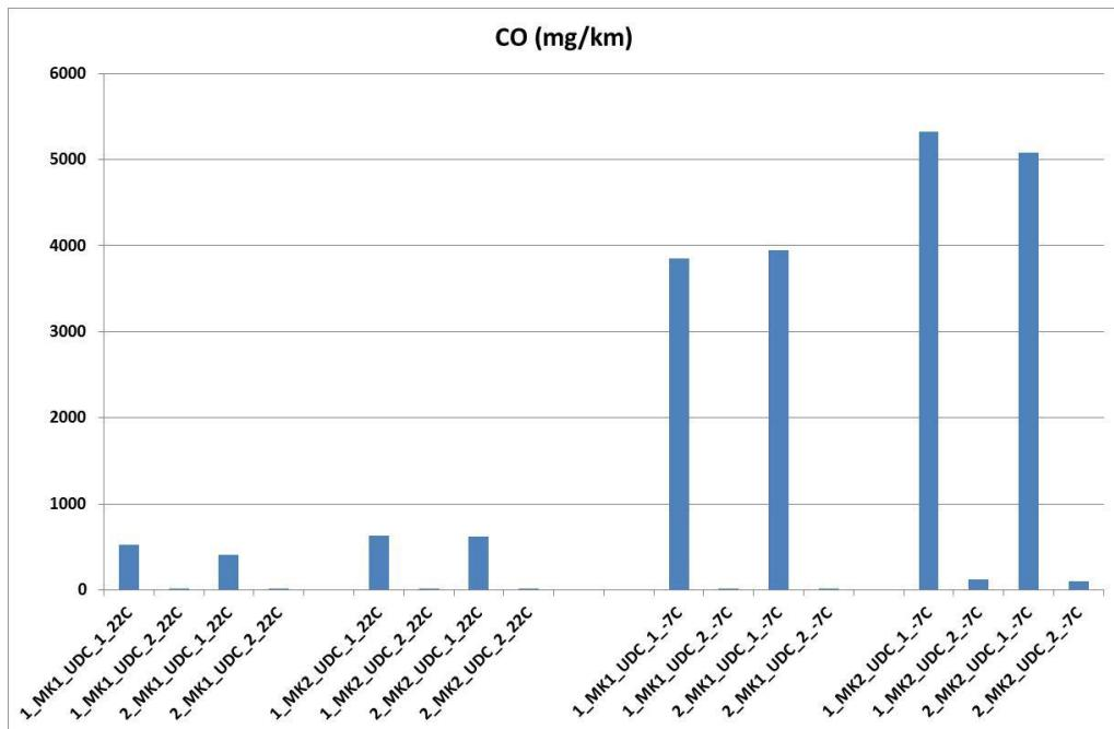
Use of MK2 seems to show higher CO emission compared with use of MK1. By comparing the graphs from the modal measurements (see below) MK1 and MK2 show similar behavior. After reaching full catalytic activity (about 30 second at 22 C and about 60 second at – 7 C) the CO emissions are close to zero for both fuels.
