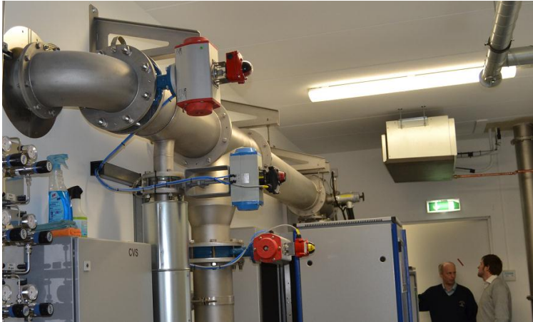
Above, CVS Dilution tunnel is showed
