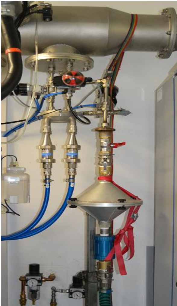
Above, Filter holder for solid phase PAH and for gas phase PAH (blue). Up to left is the tube for aldehyde sampling probes showed.
