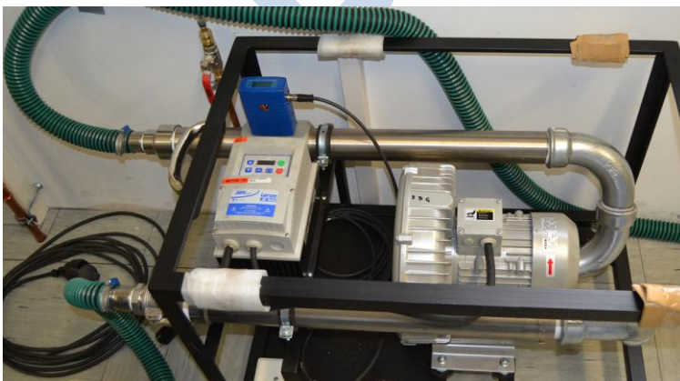
Above, pump and flow meter for sampling PAH-sampling.
