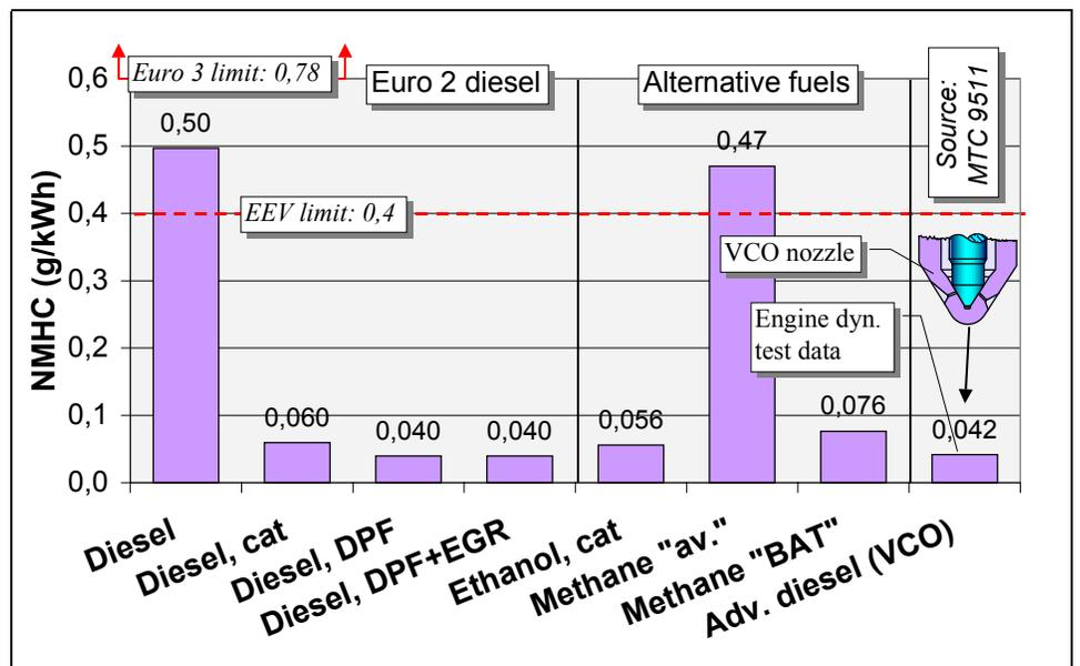
Figure 23. Impact of advanced technology on NMHC emissions (calculated data & test data)
