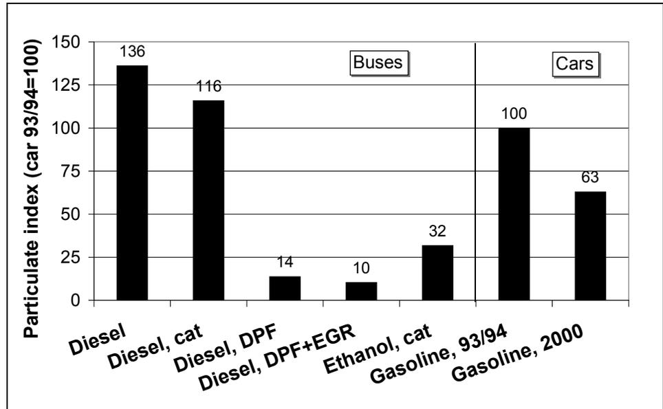
Figure 18. Particulate emissions (buses vs. cars)
