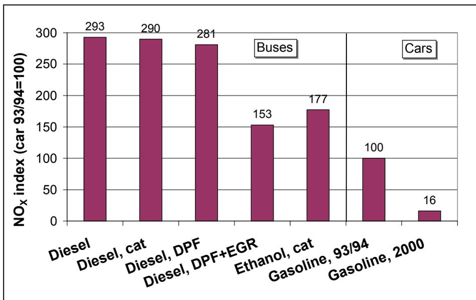
Figure 17. NO<sub>x</sub> emissions (buses vs. cars)
