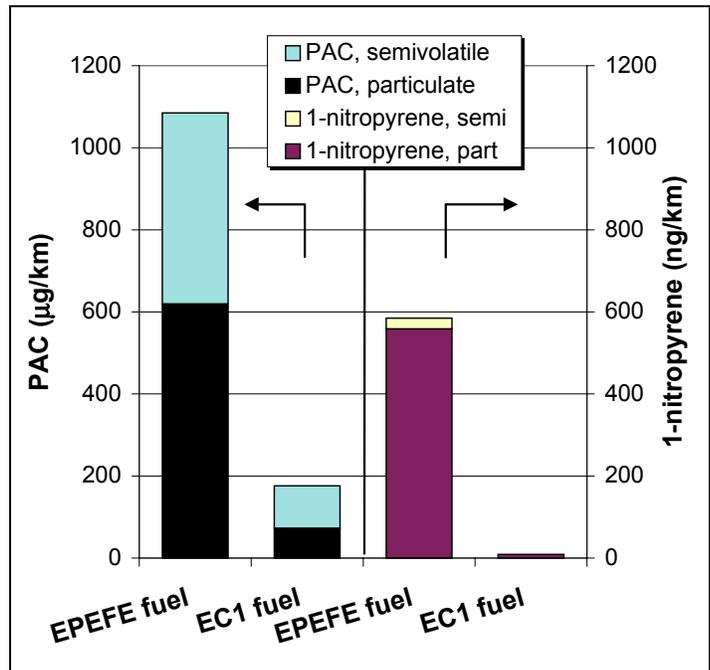
Figure 21. PAC and 1-nitropyrene emissions from two different diesel fuels qualities (HD truck)
