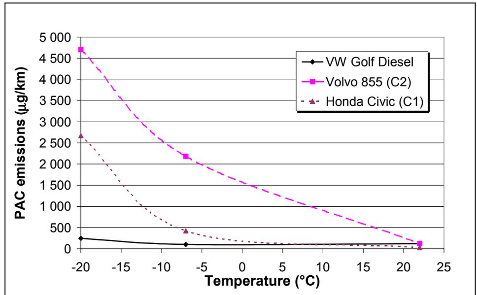
Figure 20. PAC emissions at various temperatures for three passenger cars
