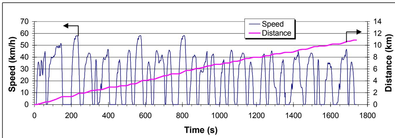
Figure 1. The Braunschweig city bus driving cycle for tests on chassis dynamometer
