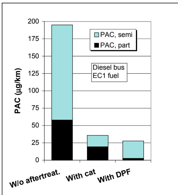
Figure 22. PAC emissions without aftertreatment, with catalyst and with particulate filter (EC1 fuel)
