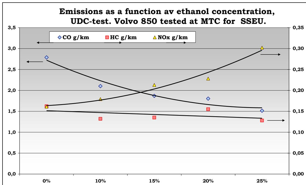
**Figure 16. Regulated emissions as function of ethanol concentration**
