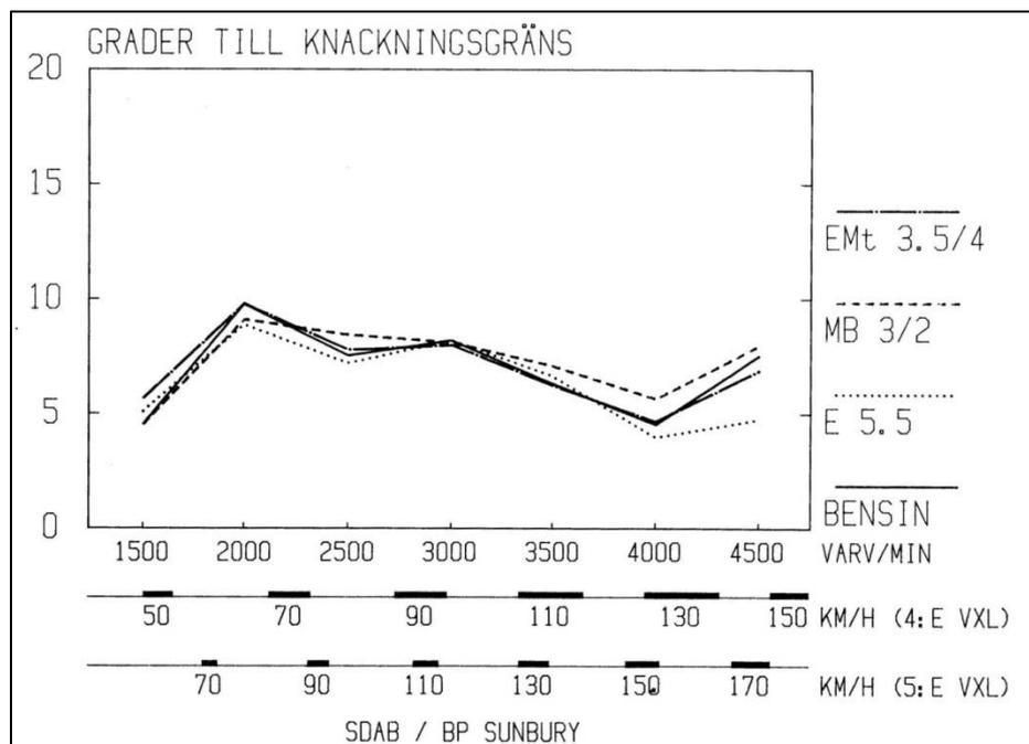
In the Figure 5, the full load knock limit at speeds from 1 500 to 4 500 rpm is shown. All the fuels perform well, the methanol/isobutanol being a little better in the high speed range and ethanol a little worse. Differences, however, are small (SDAB, 1984).
