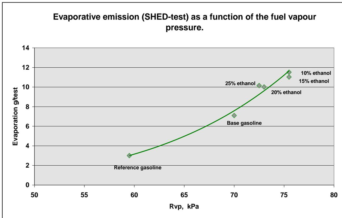
**Figure 15. Evaporative emission (SHED test) as a function of vapour pressure**
