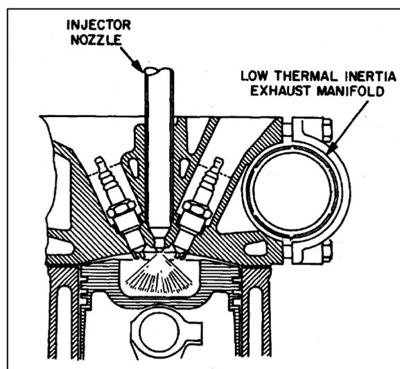
Figure 22. Cross section of the PROCO engine
