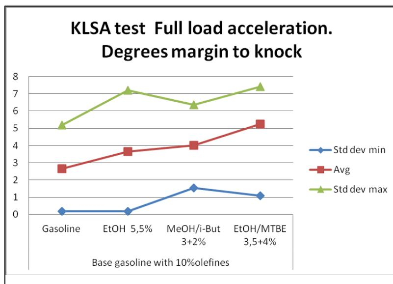
**Figure 7.** KLSA test Full load acceleration. Crank angle degrees margin to knock.
