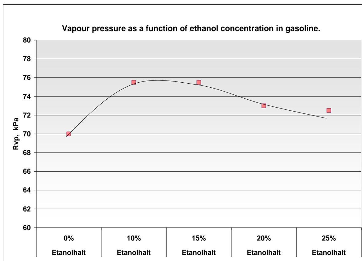
**Figure 14. Vapour pressure as a function of ethanol content**
