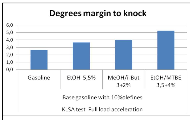
**Figure 6. Crank angle degrees margin to knock**
