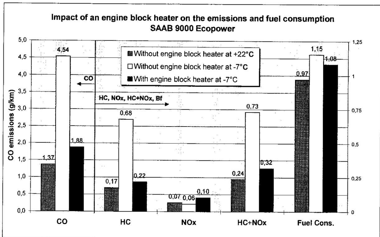
**Figure 12:** Emissions from a SAAB Ecopower with and without an engine block heater
