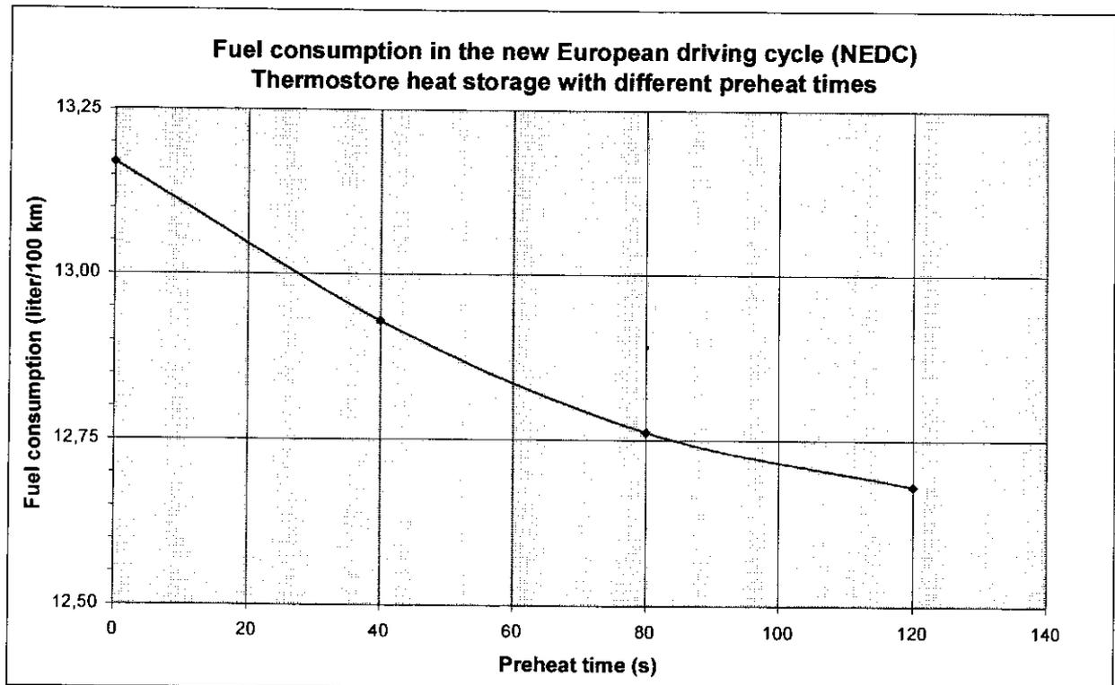
**Figure 10:** *Fuel consumption with different preheat times*
