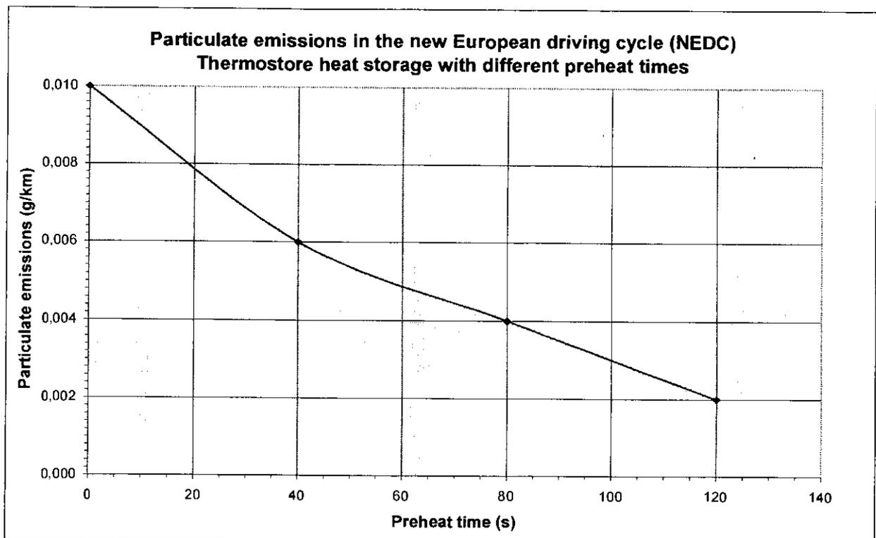
Figure 8: Particulate emissions with different preheat times
