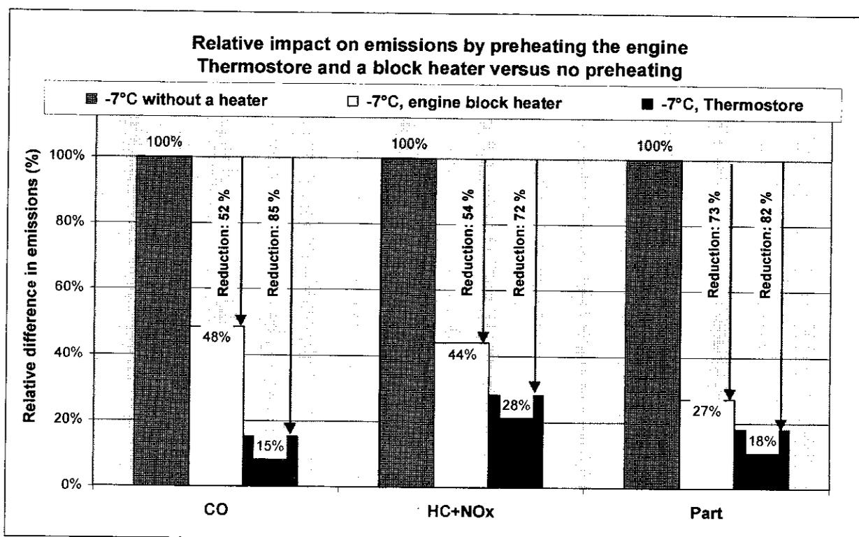
**Figure 6:** Summary of the emission potential with different preheating
