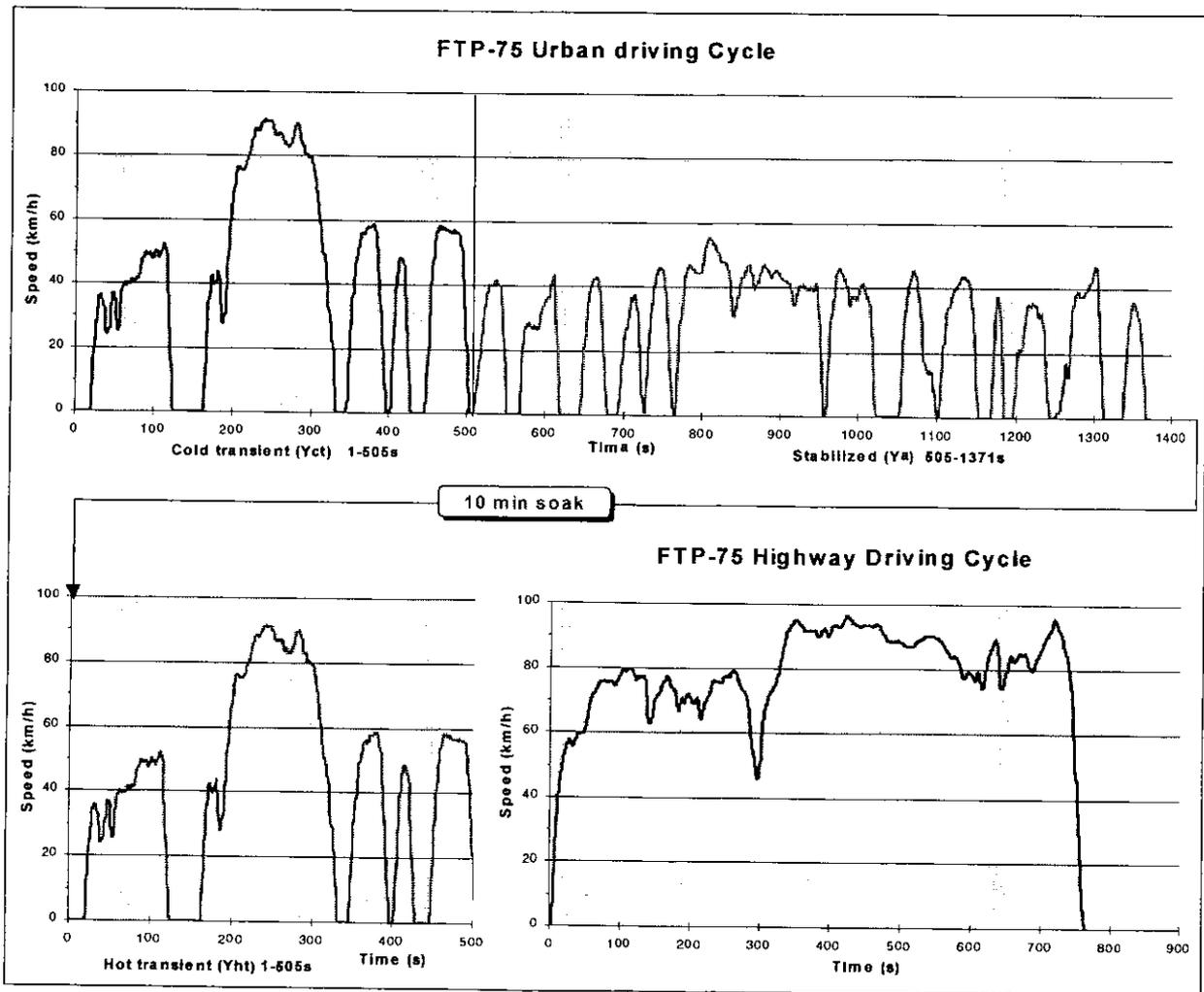
Figure 4: The FTP-75 driving cycle
