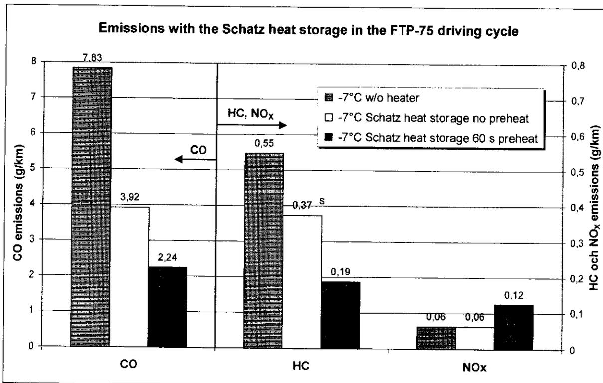
**Figure 13:** Emissions with the Schatz heat storage
